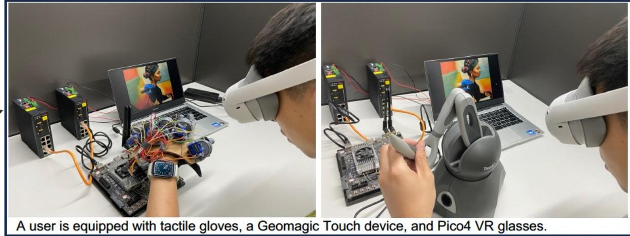
A user is equipped with tactile gloves, a Geomagic Touch device, and Pico4 VR glasses.
